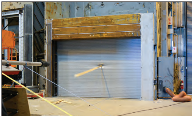
The missile impact test proves the ability to withstand wind-borne debris from a hurricane or tornado.
