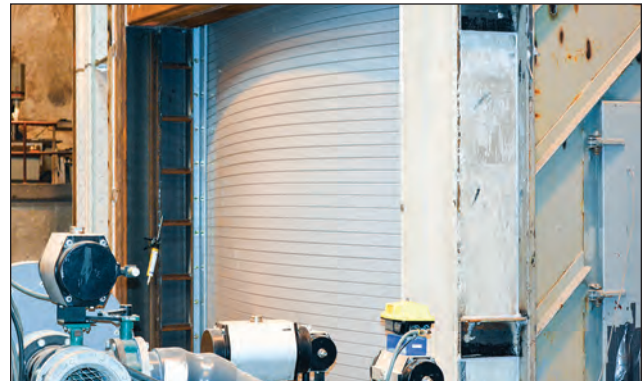
The SafeSpace 500 was subjected to both a positive and negative pressures equal to 1.2 times the 255 mph design wind load.
